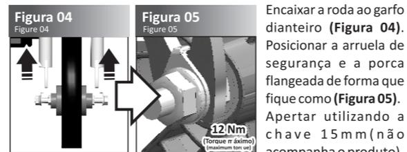
Insert the wheel to the front fork (Figure 04), Position the security washer and the flange nut as shown in (Figure 05). Tighten it using a 15mm wrench (Not included with the product).
